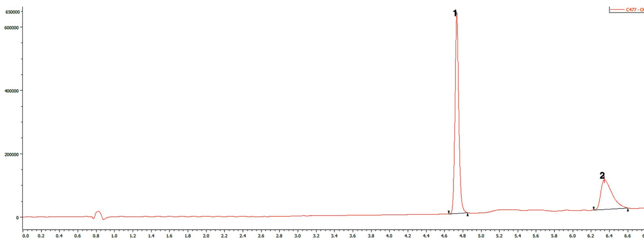
Fig. 2 LC-UV chromatogram (198 nm) of a mixed sample containing 54% phenacetine (peak 1) and 46% cocaine (peak 2)
